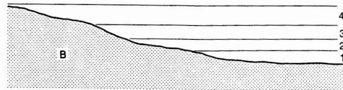
Fig. 08 Cross-section showing onlap of successive beds 1–4, each resting partly on older basement B.
