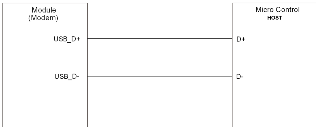
Figure 3-20 Recommended circuit of USB interface
